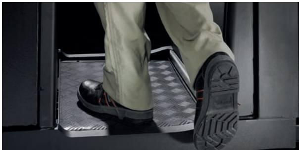
BT Optio's low step-in height reduces the strain of repeatedly stepping into and out of the truck. The floor is suspended to reduce vibration
