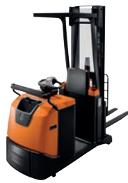
L-series, CB version, 1200 kg Picking height: 0 m–1,6 m Max. lift height: 4,1 m
