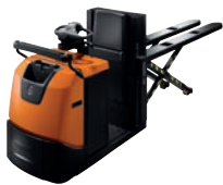
L-series, 1000 kg–2500 kg Picking height: 0 m–2,6 m
