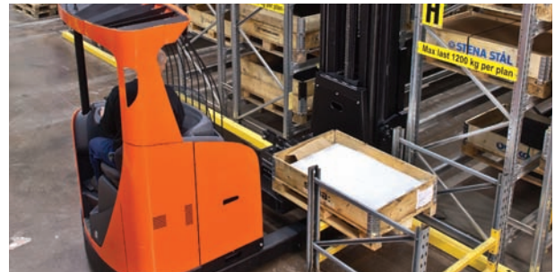
The VRE125SF's shuttle forks allow the narrowest aisles, for maximum use of space
