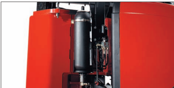
The BT Advanced Lifting System reduces energy consumption by minimising the power required from the lifting motor
