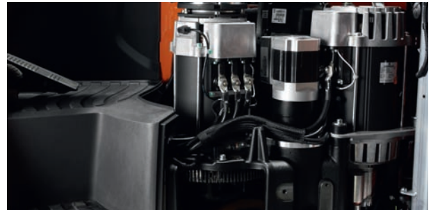
The AC motors are brushless, reducing maintenance requirements
