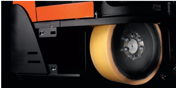
The size of the drive-wheel on the BT Vector R-series has been substantially increased, reducing wear and improving the ride quality
