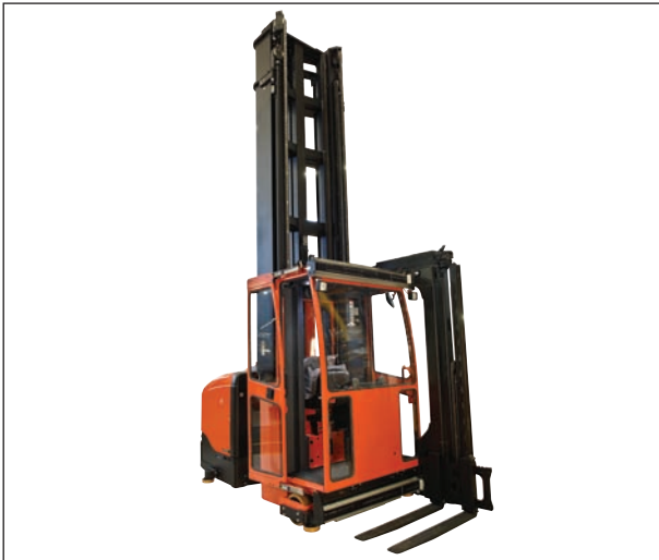
The space-saving benefits of Advanced VNA are particularly relevant in cold store environments. The BT Vector A-series is available with full cold store protection and a heated drivers cab.
